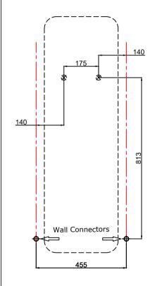
Fix the wall mounting apparatus on the wall as illustrated.
