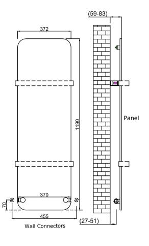
Determine the position of the product according to the water inlet - outlet dimensions stated in the figure.
